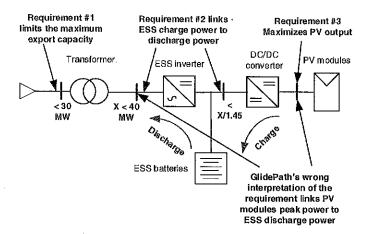
PV modules can only produce DC electric current; thus there simply is no way to link an AC MW rating to the amount of PV modules, or in other words to what GlidePath refers to as Mega-Watt peak capacity (MWp).
