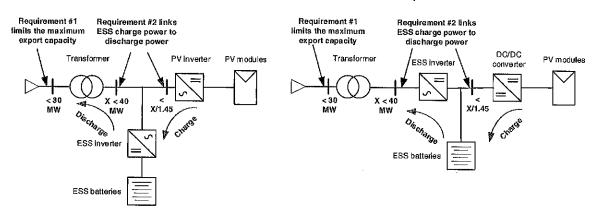
Regardless of the design, it is the Power Conversion System ("PCS") of the PV system, either the PV inverter or DC/DC converter, that controls the power flow from the PV arrays to the ESS battery modules. Consequently, the PV charging system MW rating is equal to the maximum power allowed by the inverter (in AC-coupled solutions) or the maximum power allowed by the DC/DC converter (for DC-coupled solutions).
