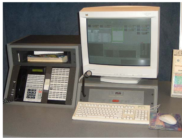
Guam's Enhanced 911 Emergency Reporting System Console
