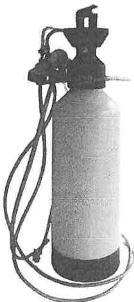
Figure 69 — PPU 1 portable test rig
